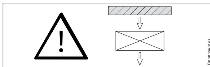
The appliance is designed for siting in front of a wall. Observe the minimum clearances. If the appliance is installed in an open space or on a roof, protect the air intake side. Do this by erecting a wall to shield it against the wind.
