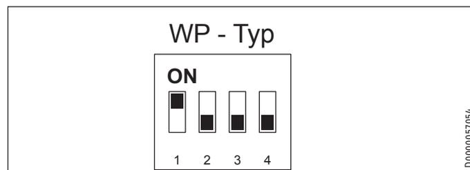
► Check whether the DIP switch is set correctly.
