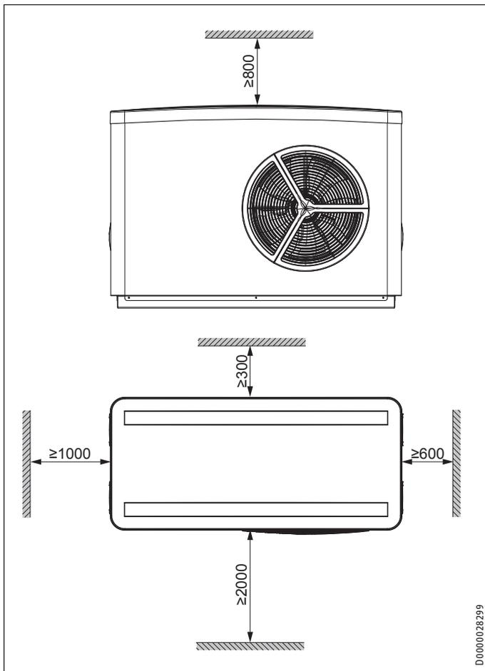
► Maintain the minimum clearances to ensure trouble-free operation of the appliance and facilitate maintenance work.
