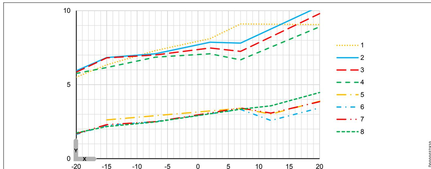
X Outside temperature [°C]    1 max. W65                      3 max. W45                      5 min. W65                      7 min. W45
