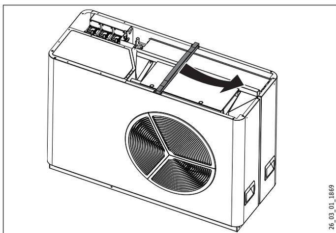
► Remove the bracket highlighted in grey.
