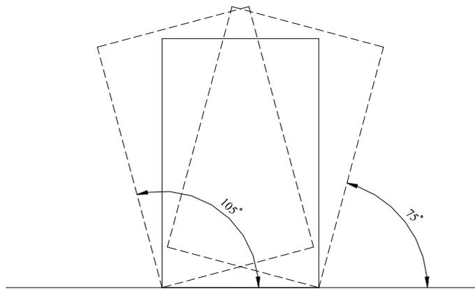
Figure 2- 1 The tilt angle of the unit
