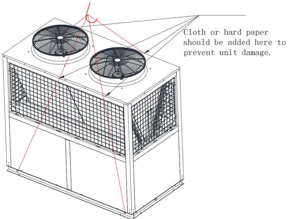
Figure 2- 3 Lifting of the unit
