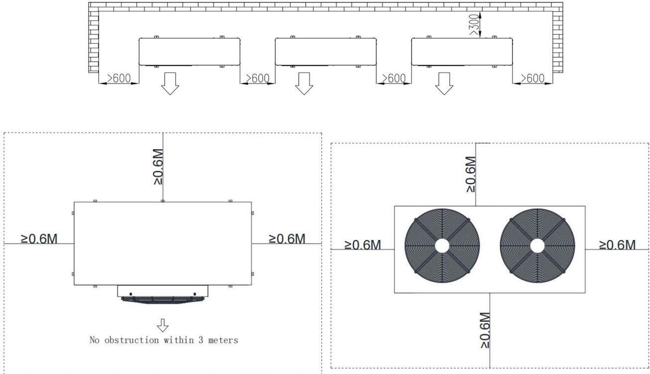
Figure 2- 4 Recommended installation spacing diagram for unit installation
